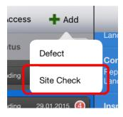
Compared to "Defect" Record, "Site Check" has less information which is used for a quick site inspection to record ongoing progress of construction.
